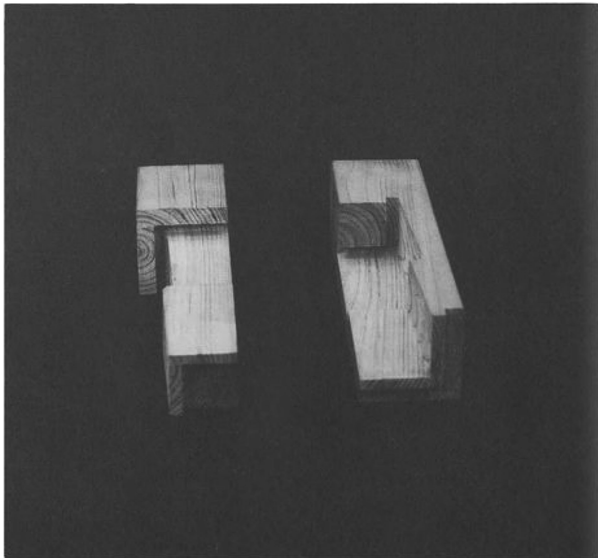
③ A shift in axial direction opens a gap between the middle drops.
