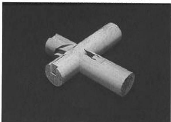
3 The girder nose (B-1) is rotated at 90 degrees from its previous position.
